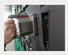
**Easy Maintenance:** Support full front maintenance, featuring hot-plug modules and cable-free connection.
